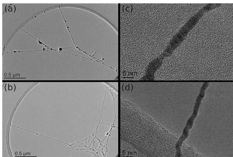
**Figure 1.** Transmission electron microscope JEOL JEM-2100 images of gold and platinum nanowires deposited on a carbon-coated copper grid. Fragments of nanowire bundles in the vicinity of 3 mm-holes in the grid: (a) gold; (b) platinum. The structure of the nanowires at high resolution: (c) gold; (d) platinum.
