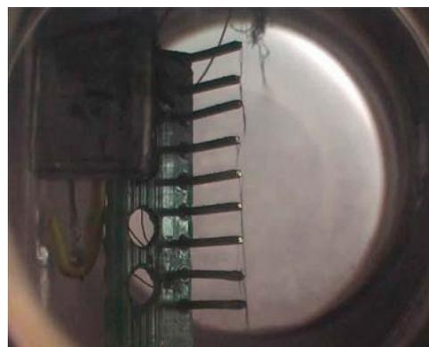
**Figure 4.** The photo of platinum nanowire bundles grown in superfluid helium made through cryostat windows. The nanowires preferably pinned to the tips of adjacent electrodes closing the electrical circuit.
