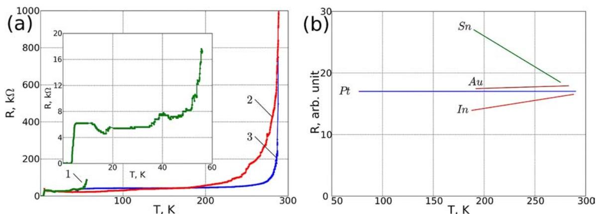
**Figure 2.** Electrical resistance,  $R$ , of the 1.4 mm long bundles of nanowires versus temperature: (a) 1 – mercury; 2 – gold (in the figure scale, the curve for platinum almost coincides with that for gold); 3 – tin (dependence for mercury is in 5:1 scale); the inset shows  $R$  versus  $T$  dependence for mercury in real scale. (b) The temperature dependences of resistance for annealed bundles of nanowires made of gold, platinum, tin, and indium (see text for the details of annealing).
